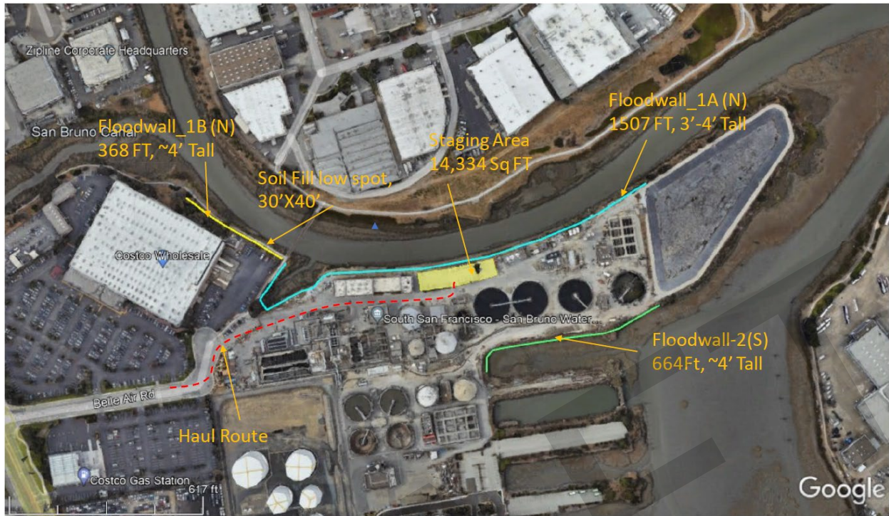
Figure 3. Floodwall alignment on main property of WQCP.
